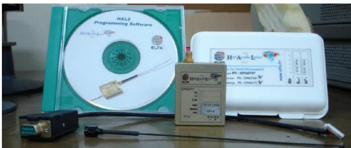
Fig. 20. *Kit completo do transmissor UHF ELTA HAL-2.*
