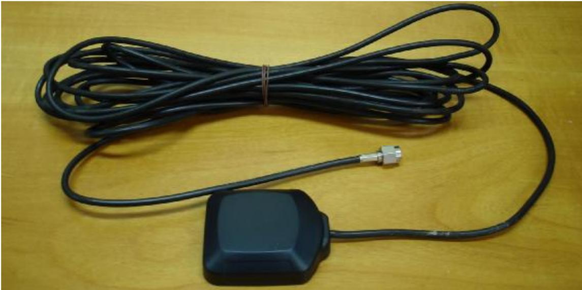
**Fig. 18. Antena do receptor GPS Trimble Lassen iQ.**
