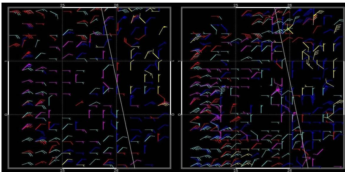
**Figure 1:** Comparison between the wind field resulting when using target windows with sizes 10x10 (left) and 8x8 (right). Vectors blue and light blue are 6.3  $\mu\text{m}$  and 10.8  $\mu\text{m}$  respectively. Other colors as difference ranges, yellow is 5 to 12 K, pink is -5 to 2 K, red is 0 to 7 K.
