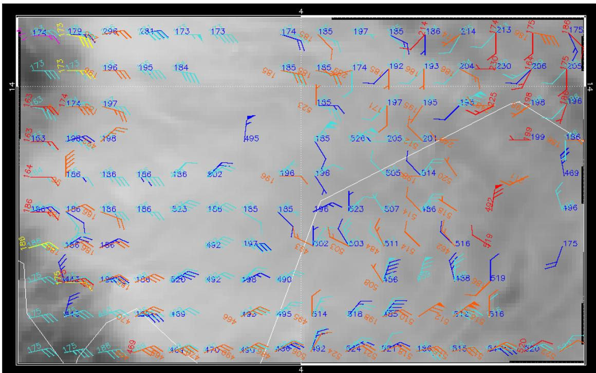
**Figure 3:** Wind shear captured by 8.7  $\mu\text{m}$  – 13.4  $\mu\text{m}$  channel difference of Meteosat 8. In background we have a image from 10.8  $\mu\text{m}$ . Blue and light blue are 8.7  $\mu\text{m}$  and 13.4  $\mu\text{m}$  SEVIRI channels, the other colors are the BTM range, red: -10 to -3 K, orange: -5 K to 2 K and yellow: -15 to -8 K.
