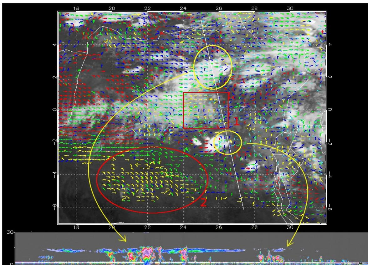
**Figure 4:** Wind vectors from 7.3-12 μm channel difference plot above a 10.8 μm SEVIRI image. The straight white line represent the Cloudsat measurement for around 12:45 utc. In the bottom we can see the Cloudsat CPR radar measurements (raw echo power return), the left side represent the north west measurement and right the south east.
