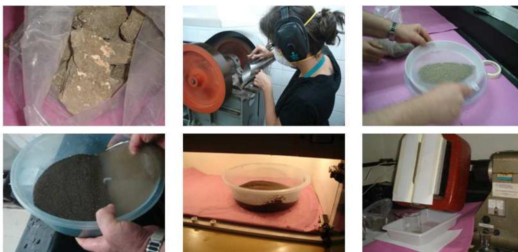
Figure A.7 – Rock processing stage
