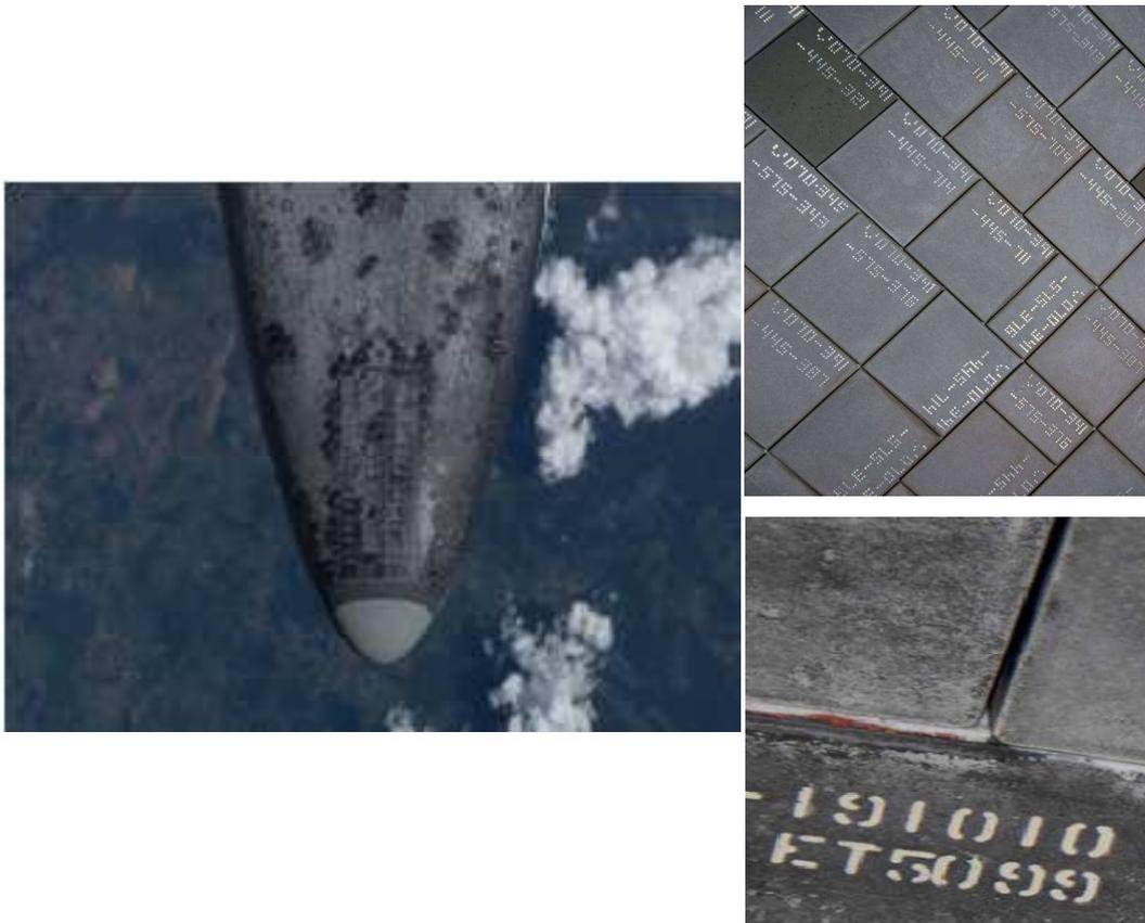
Figure 1.2 - Drawing illustrating the tile configuration of the Space shuttle Orbiter.
