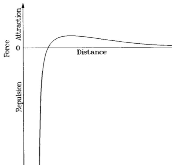
Figure 2.3 - Typical intermolecular force field.
