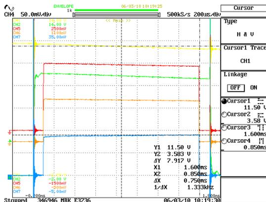
Figure 2: Waveforms. Cathode voltage (115kV, 1.7ms-long, yellow), collector current (133A, 1.7ms-long, green), RF output from the two ports (10.2MW in total, 1.5ms-long, red and orange).
