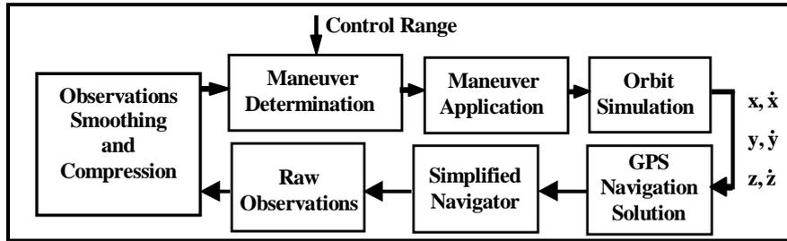
Figure 2. Block Diagram of the Autonomous Control System
