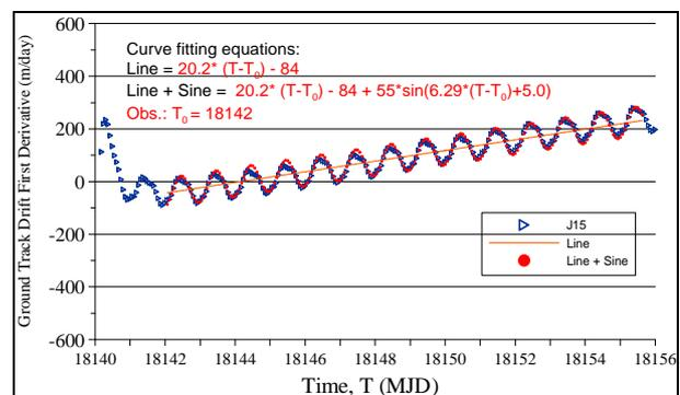
Figure 1.b - Filtering Equations for  $\dot{D}$
