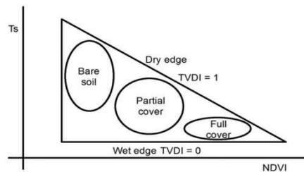
**Figure 2. Schematic representation of the Evaporative Triangle, given by the relationship between surface temperature ( $T_s$ ) and normalized difference vegetation index (NDVI); Source: Shirmbeck et al. (2018).**
