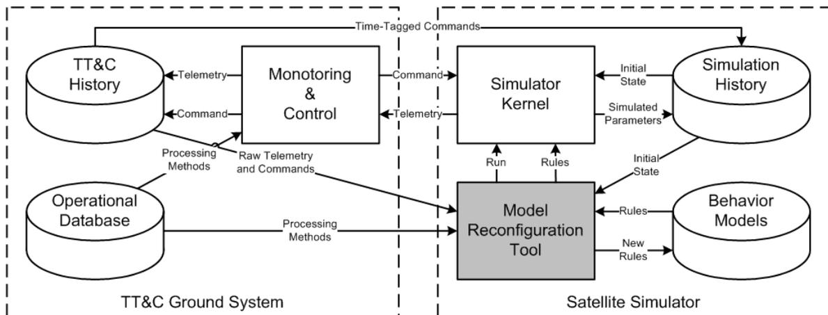
Figure 2. Automatic simulator model reconfiguration software architecture.
