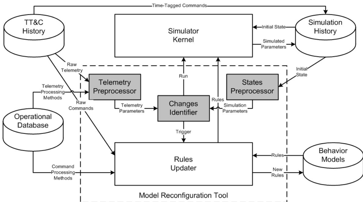
**Figure 3. Software architecture for comparative analysis between telemetry and simulation parameters.**
