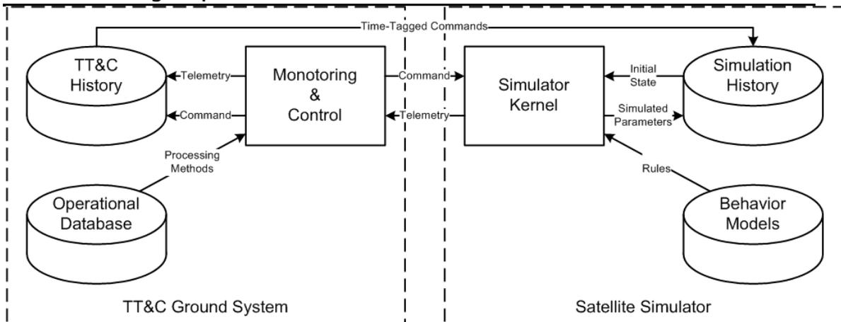
Figure 1. Operational simulator software architecture.
