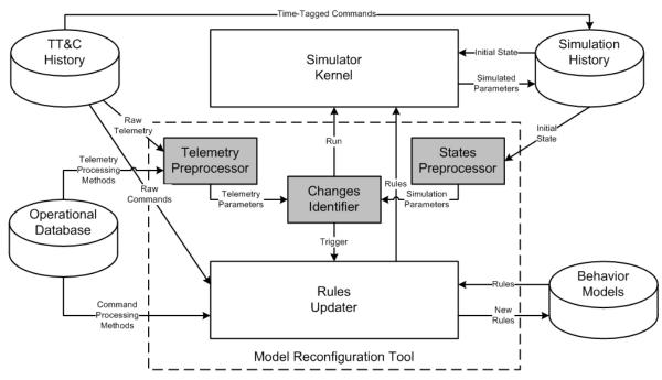
Figure 3. Software architecture for comparative analysis between telemetry and simulation parameters.
