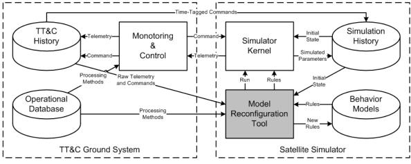
Figure 2. Automatic simulator model reconfiguration software architecture.
