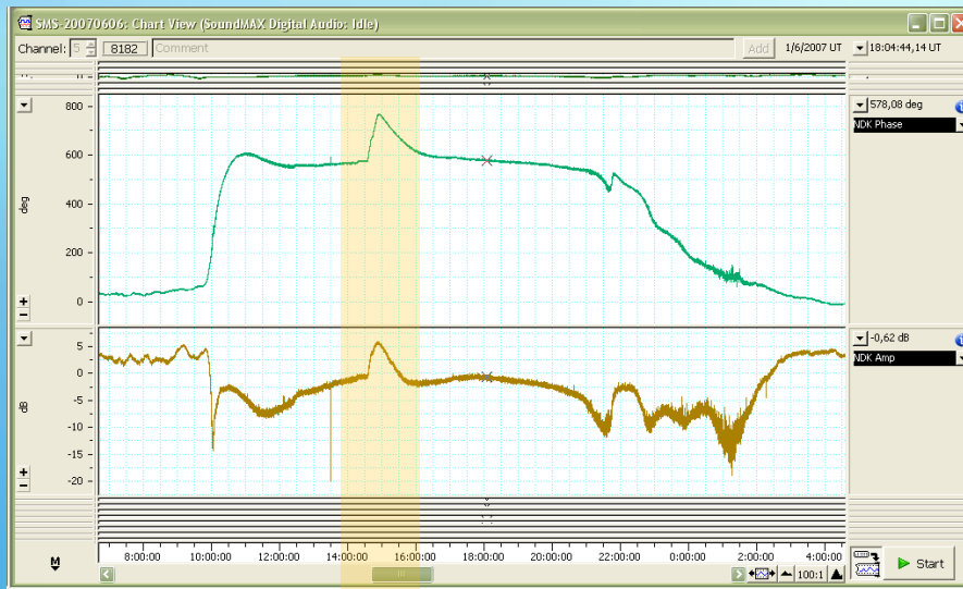
M2.8-Class Solar flare observed at SSO with the VLF SAVNET Station on June 01, 2007.
