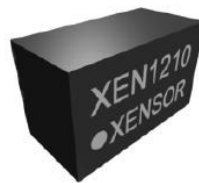
Fig. 1 SFN8 Package of XEN - 1210 - Xensor Integration – XI. The dimensions are 2x2,4x4 mm [4] .
