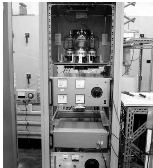
Fig. 27. Left: Schematic of the improved monotron power supply (10 kV, 3×8 A) using three tetrodes in parallel. Right: Picture of the monotron high-voltage and high-current power supply
