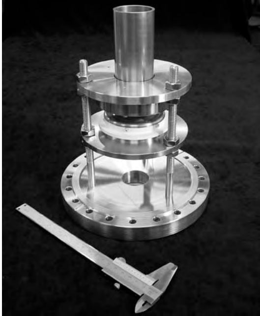
Fig. 25. Left: Full monotron mounted on a CF150 vacuum flange. The assembly includes the injection electron gun shown in the middle part of the picture, and the resonant cavity coupled through a circular hole to the TM-mode output waveguide shown in the top part of the picture. Right: Test of the high-voltage and high-current power supply with single tetrode.
