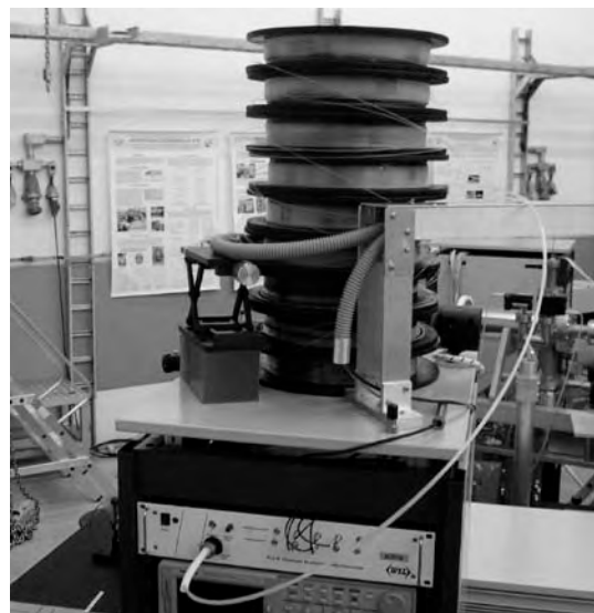
Fig. 10. Above: Light collection optics of the 10-channel Thomson scattering (TS) diagnostic. Right: Stack of fiber optics reels forming the delay line of the 10-channel TS diagnostic.
