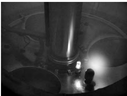
Fig. 29. Left: Picture showing the glow discharge electrode (bottom of the image) and the preionization filament. Right: Residual gas analysis just after a vacuum break (top) and after about 60 h of baking (bottom). The analysis after baking indicates removal of N 2 ( m/q=28 ) and O 2 (32), traces of H 2 (2) and CO (28), but still considerable amounts of water.
