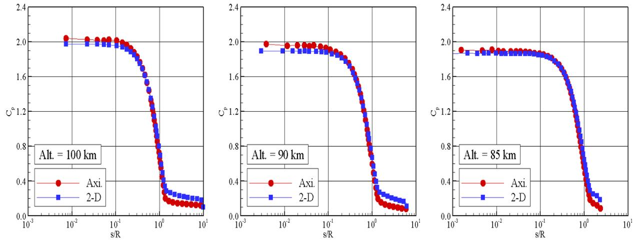
Figure 7. Distribution of pressure coefficient  $C_p$  along the capsule surface for altitudes of (a) 100 km, (b) 90 km, and (c) 85 km.
