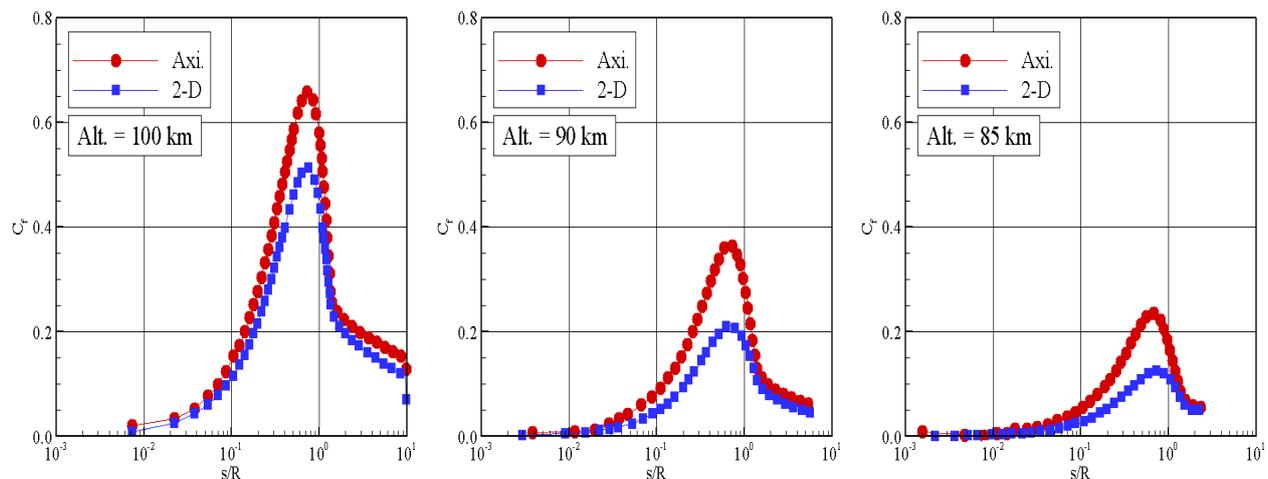
Figure 9. Distribution of skin friction coefficient  $C_f$  along the capsule surface for altitudes of (a) 100 km, (b) 90 km, and (c) 85 km.
