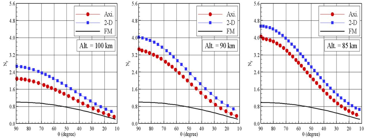
Figure 4. Distribution of the dimensionless number flux  $N_f$  along the capsule surface as a function of the body slope angle  $\theta$  for altitudes of (a) 100 km, (b) 90 km, and (c) 85 km.
