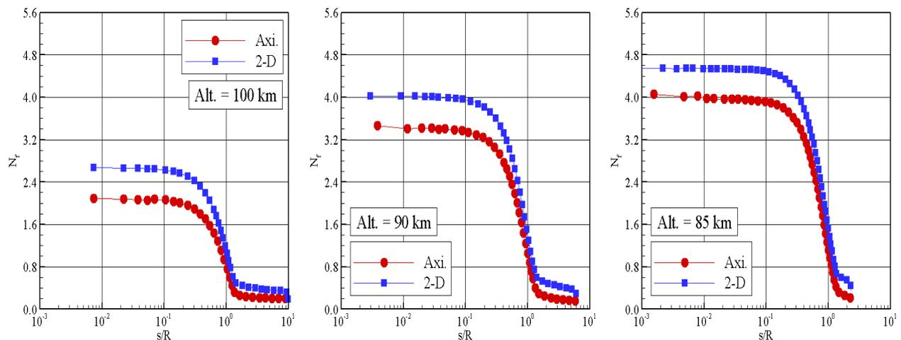
Figure 3. Distribution of the dimensionless number flux  $N_f$  along the capsule surface for altitudes of (a) 100 km, (b) 90 km, and (c) 85 km.
