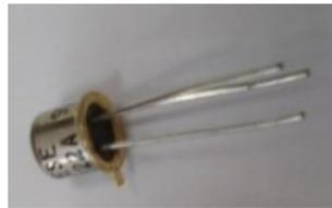
Figura 2. Transistor 2N2222A.
