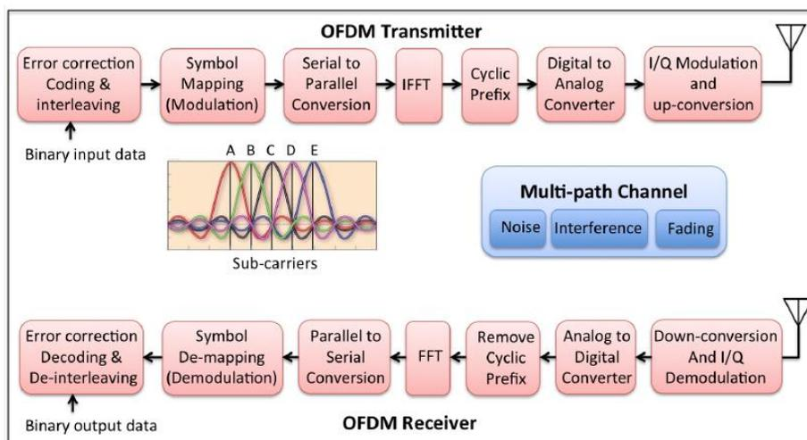
**Figure 4. OFDM overall communication system.**
