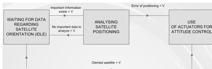
**Figure 9. State transition diagrams for product in operation.**
