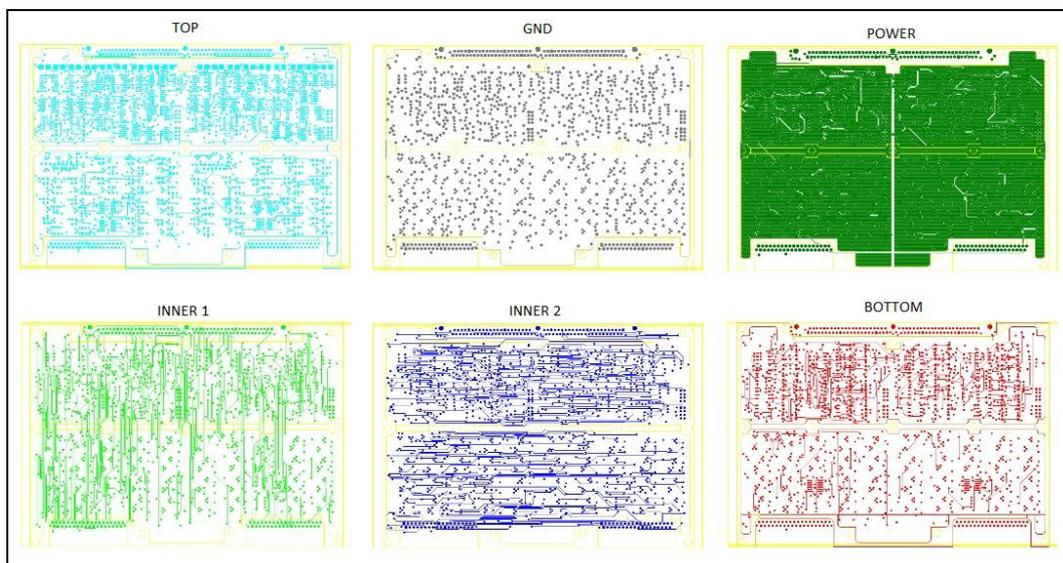
Figure 3. The 6 signal layers of the PCB.
