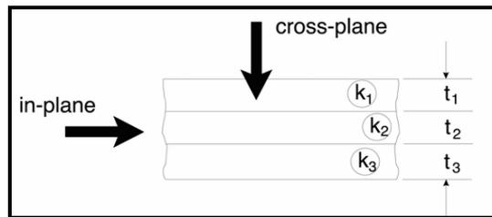
Figure 5. Basic conductivity definition in laminated substrate.
