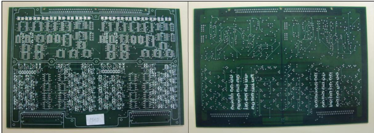
Figure 2. Multi-layered PCB for space applications (top/bottom photos).
