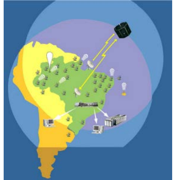
Figure 1. ITASAT System related to data collection, where the ITASAT-1 satellite plays a very important role to the continuity of the Brazilian Environmental Data Collection System.
