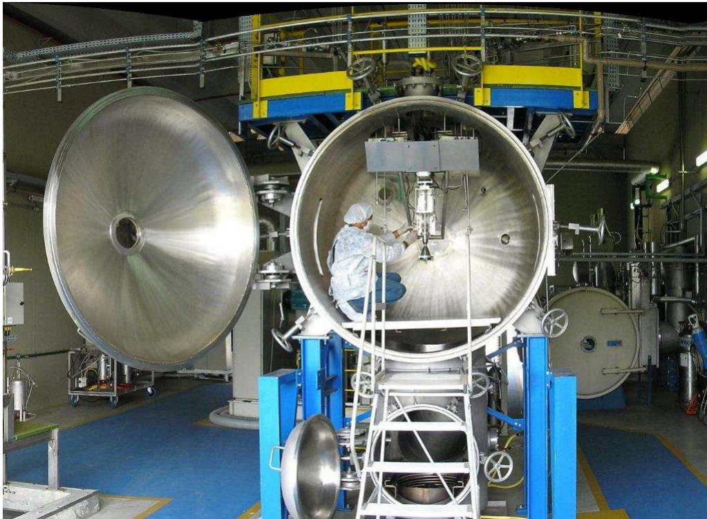
Figure 5. Test Facilities with Simulate Altitude (BTSA) at LCP/INPE
