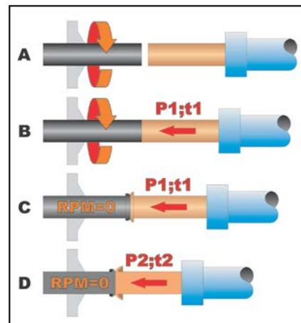
FIGURE 2 – EQUIPMENT OF ROTARY FRICTION WELDING [2]
