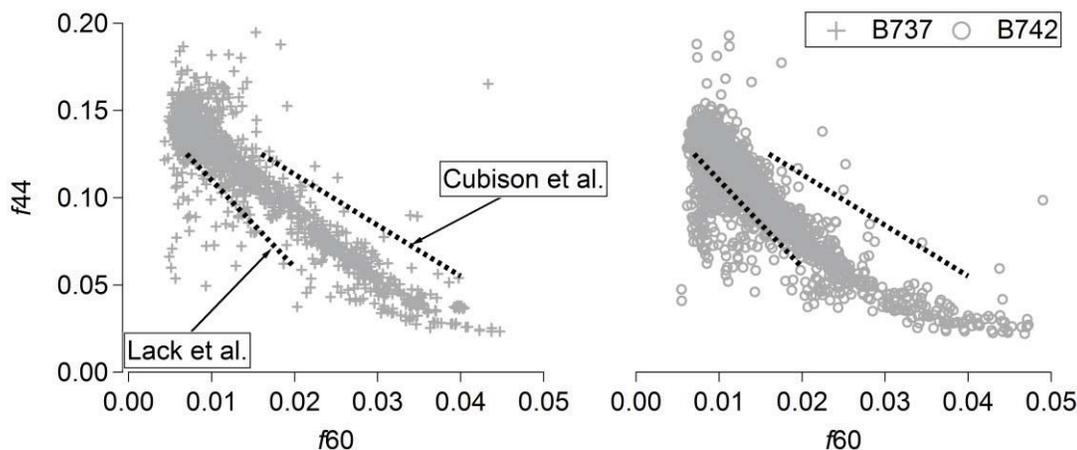
**FIGURE 2.** Relationship between  $f_{44}$  and  $f_{60}$  (defined below) for flights B737 and B742. The dotted lines correspond to the approximate slopes observed in Cubison et al. [1] and Lack et al. [2].
