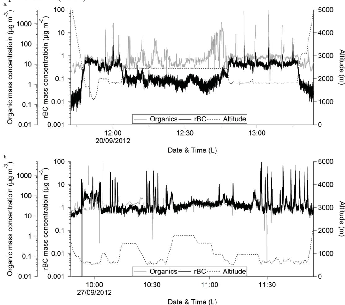
**FIGURE 1.** Time series of refractory Black Carbon (rBC) and organic aerosol for flight B737 (a) and B742 (b). The altitude of the aircraft is also shown. Note the logarithmic scales for both rBC and organic mass concentrations.
