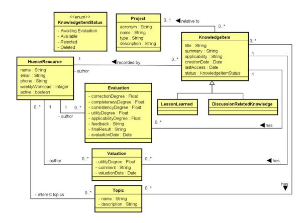
Figure 5.12 - Class diagram of KM Portal. SOURCE: Adapted from Coelho (2010)
