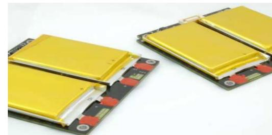
Figure 3. Clyde Space lithium polymer battery
