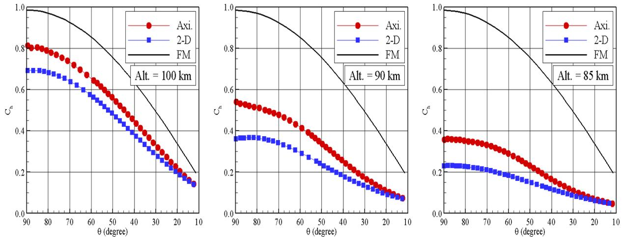
Figure 6. Distribution of heat transfer coefficient  $C_h$  along the capsule surface as a function of the body slope angle  $\theta$  for altitudes of (a) 100 km, (b) 90 km, and (c) 85 km.
