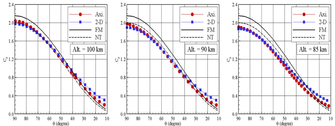
Figure 8. Distribution of pressure coefficient  $C_p$  along the capsule surface as a function of the body slope angle  $\theta$  for altitudes of (a) 100 km, (b) 90 km, and (c) 85 km.
