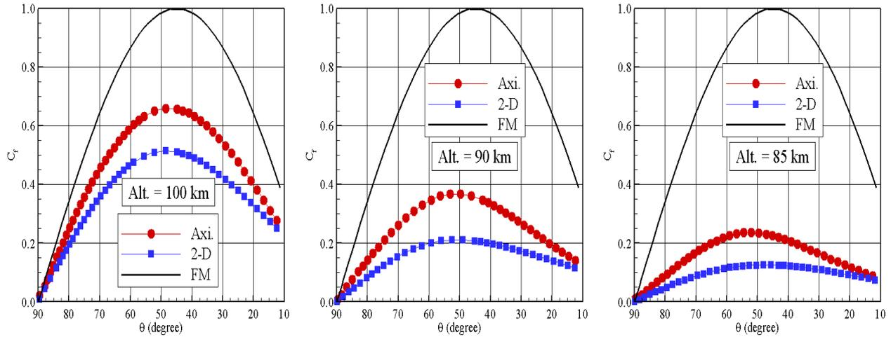
Figure 10. Distribution of skin friction coefficient  $C_f$  along the capsule surface as a function of the body slope angle  $\theta$  for altitudes of (a) 100 km, (b) 90 km, and (c) 85 km.
