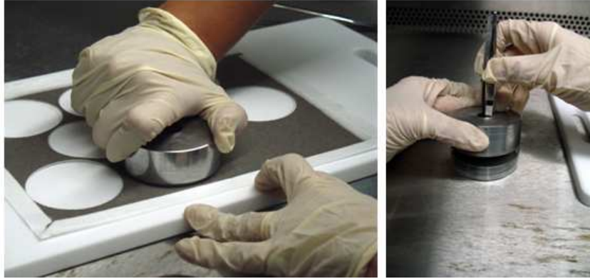
Figure 3.8 – collected glass filter been sliced to be measured.
