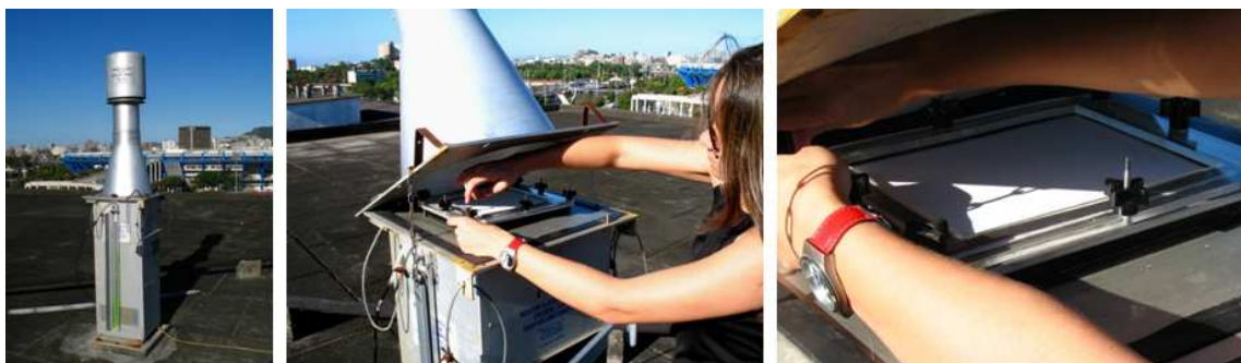
Figure 3.7 – ^7\text{Be} acquisition system installed in UERJ's campus.
