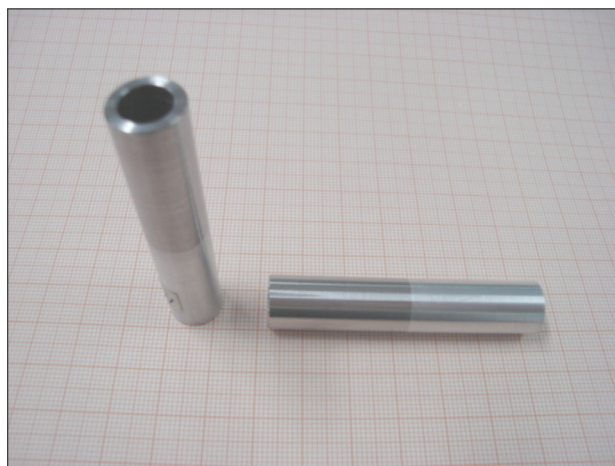
Figure 11: Joints produced by the rotary friction welding process (RFW) (dark part: AISI 304 stainless steel; clear part: AA1050 aluminum).
