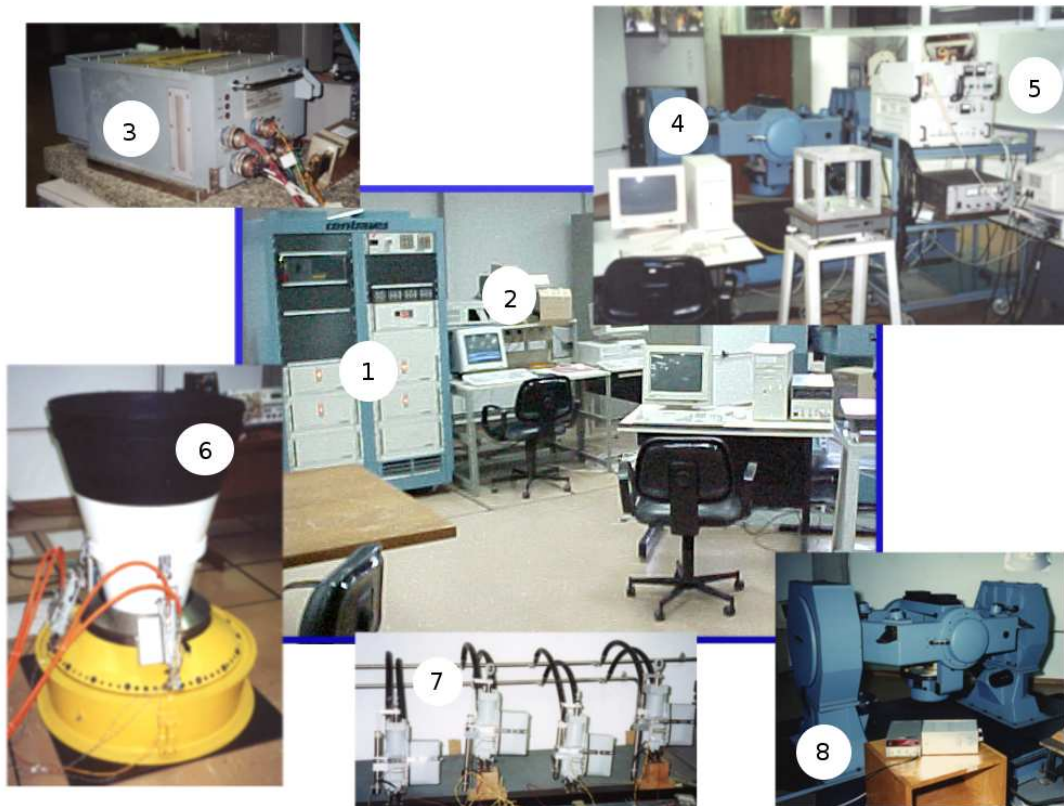
Figure 5.3 - Elements of the VLS hardware-in-the-loop simulation complex.
