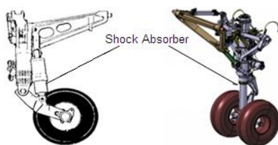
Pneumatic Shock Absorbers [Sources: Currey, 1988]
