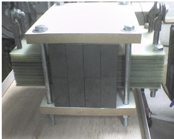
Fig. 4. Prototype of Transformer.
