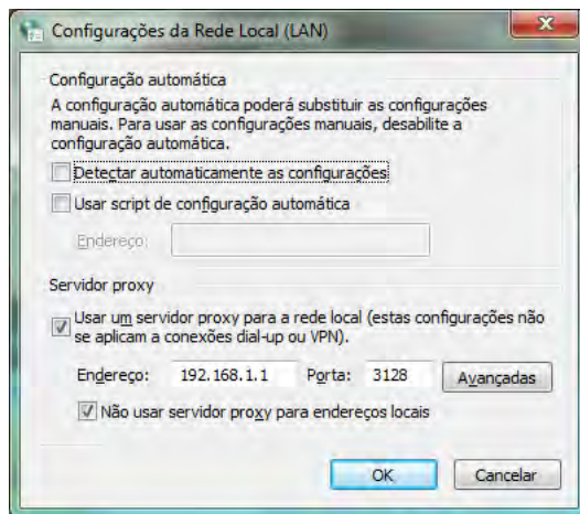
Figure A.3 - Configuration to use a proxy. (Proxy defined in the server.)
