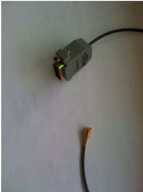
Figure 2.6 - Cable adaptation: 15-pin to SMB.
