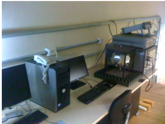
Figure 2.2 - The complete setup, the two PCs and the C-400 chassis containing the three boards. In the middle we can observe a test mass with six Piezoelectric resonators.
