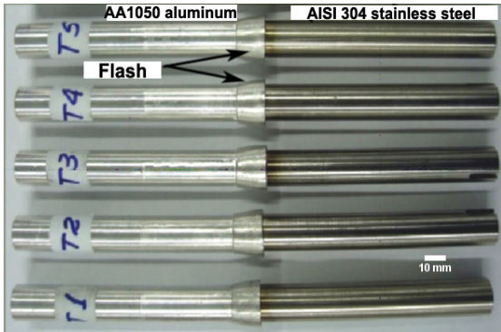
FIGURE 7 ELDED PINS BY RFW WITH THE SAME PARAMETERS
