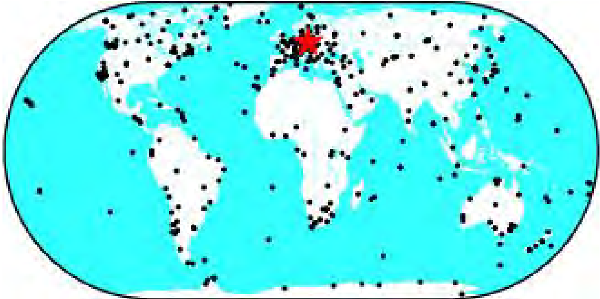
Figure 3.3: IGS network of permanent GPS tracking stations
