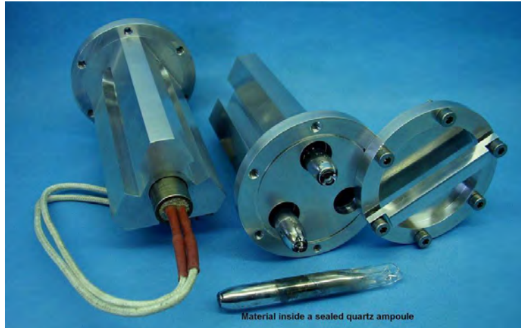
Figure 2.3 - Heater set-up showing the electric resistance and quartz ampoules.
