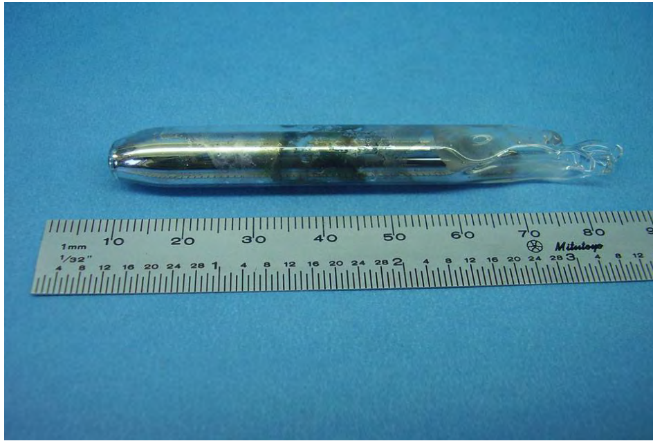
Figure 2.5 - Quartz ampoule with BiInSn alloy.
