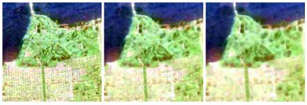
(d) Refined Lee filter I = 1 (e) Refined Lee filter I = 3 (f) Refined Lee filter I = 5
