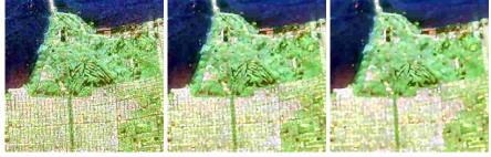
(j) SDNLM filter I = 1(k) SDNLM filter I = 3(l) SDNLM filter I = 5
