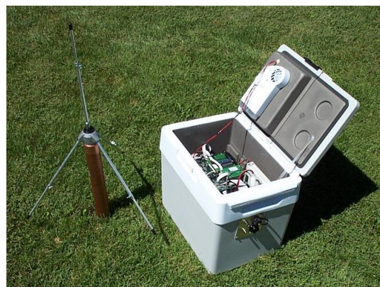
Figure 1. Portable LMA detection station
