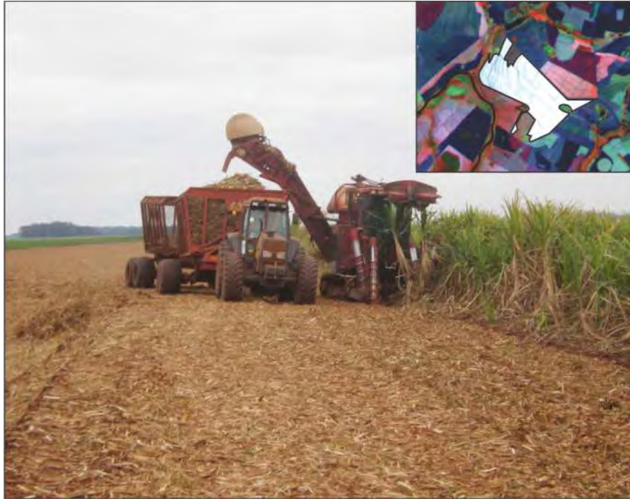
Figure 2.3 - Mechanized sugarcane harvest without BH (called GH), showing the straw remaining on the ground and highlighting (inset) its appearance in a false color composite TM/Landsat-5 image.
