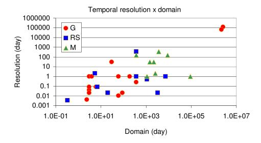
Figure 1.3 – Relation between temporal resolution and domain for ground-based (G), remote sensing (RS) and modeling (M) methods.
