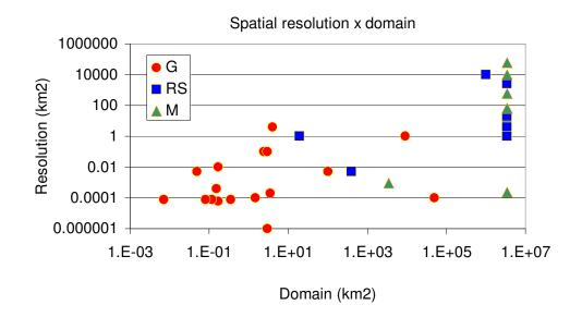
Figure 1.2 - Relation between spatial resolution and domain for ground-based (G), remote sensing (RS) and modeling (M) methods.
