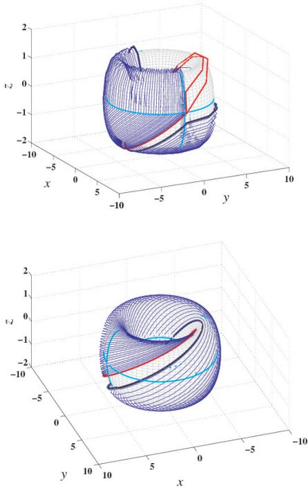
**Figure 1 – Experimentally nonlinear (top) and linear (bottom) PPT for a pair of coupled LCOs on the (1 : 1) synchronization state and in the spiking regime. Red line corresponds to the synchronized state, the black one to the initial uncoupled state and the blue ones are the orbit transients. In gray, a torus is shown with cyan lines that divide each sector.**
