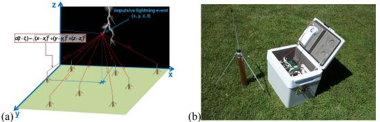
**Figure 1** – (a) Illustration of the time-of-arrival technique used by the LMA system. The times  $(t_i)$  when a signal is detected at N $\geq$ 4 stations are used to solve for the 3D source location  $(\underline{x}, y, z, t)$  of the impulsive breakdown processes associated with a discharge. (b) Portable LMA station electronic box and antenna.
