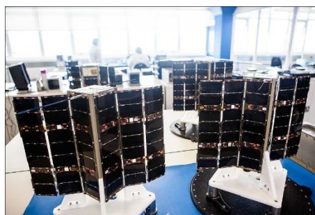
Figure 3 Triple Unit Lemur-2 Second Generation Satellites (Spire, 2019)
