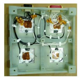
Figure 6. Heaters and thermistors placed inside the experiment assembly.
