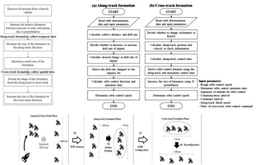
Figure 7. Change in the shape and size of the formation conducted by the four nanosats Source: Adapted from Song et al. (2021)
