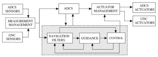
Figure 1. Block diagram illustration of the spacecraft AOCS. Source: Bong Wie et al (2014)
