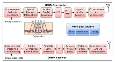
Figure 4. OFDM overall communication system.
