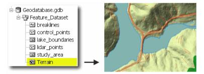
Figure 2.10 – Terrains data structure Source: ESRI (2010)
