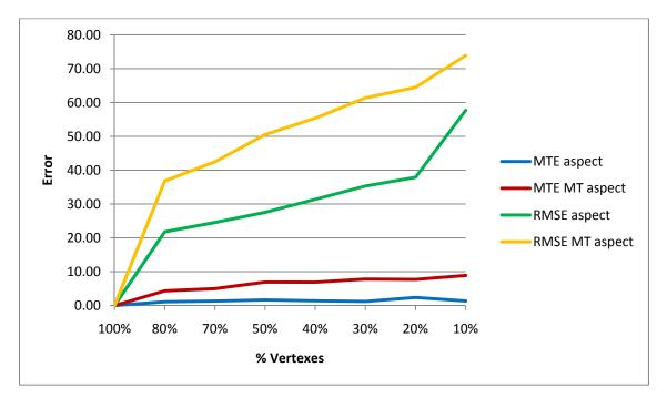
Figure 4.5 – MTE and RMSE aspect values for TIN from Mount Marcy with different number of vertexes.
