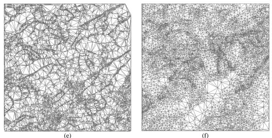
Figure 4.2 – Comparison of Multiscale TIN from Mount Marcy dataset with 80% (a) our method (b) MT, 50% (c) our method (d) MT, and 20% (e) our method (f) MT.
