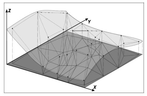
Figure 2.2 – Example of irregular grid Source: adapted from Namikawa (2003)
