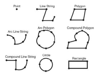
Figure 2.12 – Geometric types from Oracle Spatial Source: Murray (2009)
