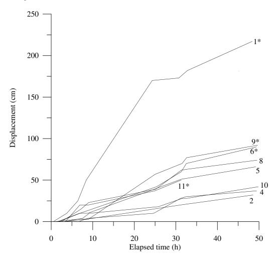
Figure 4 – Variation of smoldering front displacement as function of elapsed time for the selected logs (\*: oscillated between flaming and smoldering; 0–10, daytime; 10–22, night; 22–34, daytime; 34–46, night; 46–50, daytime) (Source: Rabelo et al., 2004).
