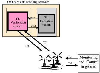
Figure 2. Telecommand verification service.
