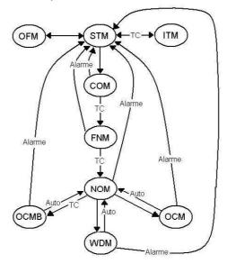
Figure 1. Transition logic of the operation modes of the PMM. INPE (2001)
