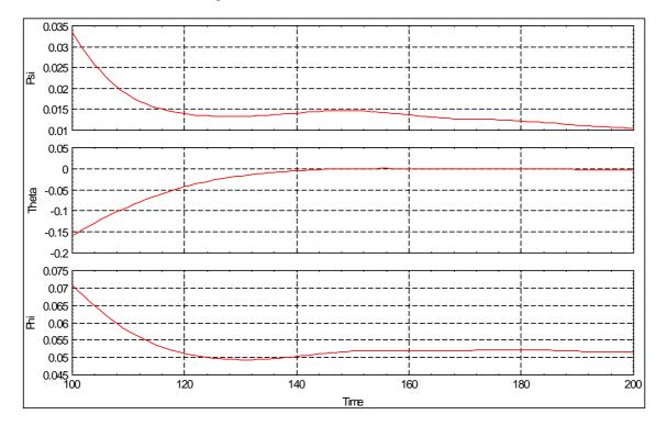
Plot 1: Attitude in degrees in all axes in referential LVLH, as a function of time in Case 1
