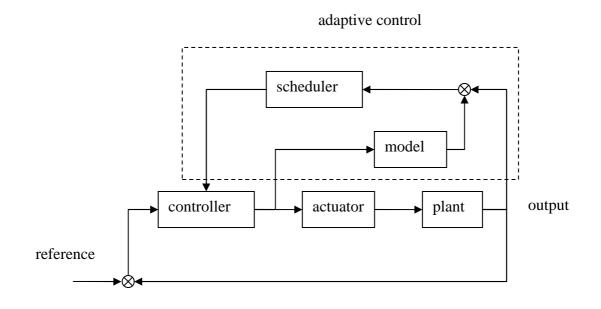
Figure 2. Block diagram of the attitude control system.
