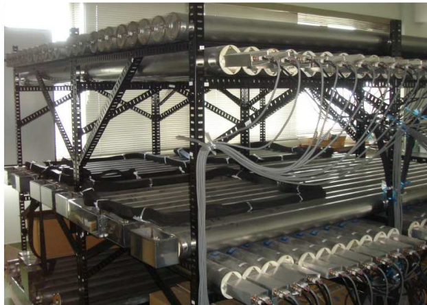
Figure 4.2. Hodoscope multidirectional muon detector installed at the University of Kuwait. Each tube is a proportional counter. The top and second layers form an upper pair, while the third and bottom layers form a lower pair. Source: Private communication from the Cosmic Ray Laboratory from Shinshu University (2010).
