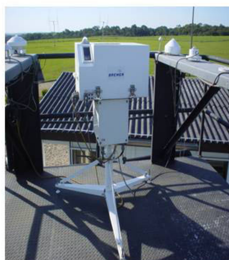
Fig. 1: Brewer Spectrophotometer installed at the Southern Space Observatory.
