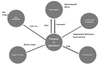
Figure 7. Context diagram for AOCS in operation.
